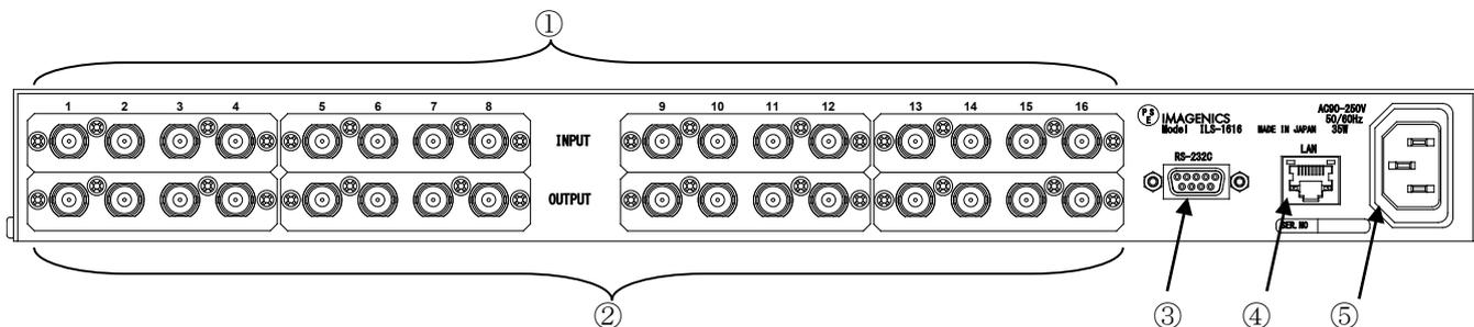
① IMG. LINK入力 (IN-1 ~ IN-16 75Ω BNC)
